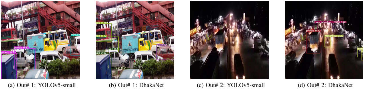
Fig. 4: Qualitative analysis between YOLOv5-small [11] and DhakaNet over two challenging test images in DhakaAI dataset
